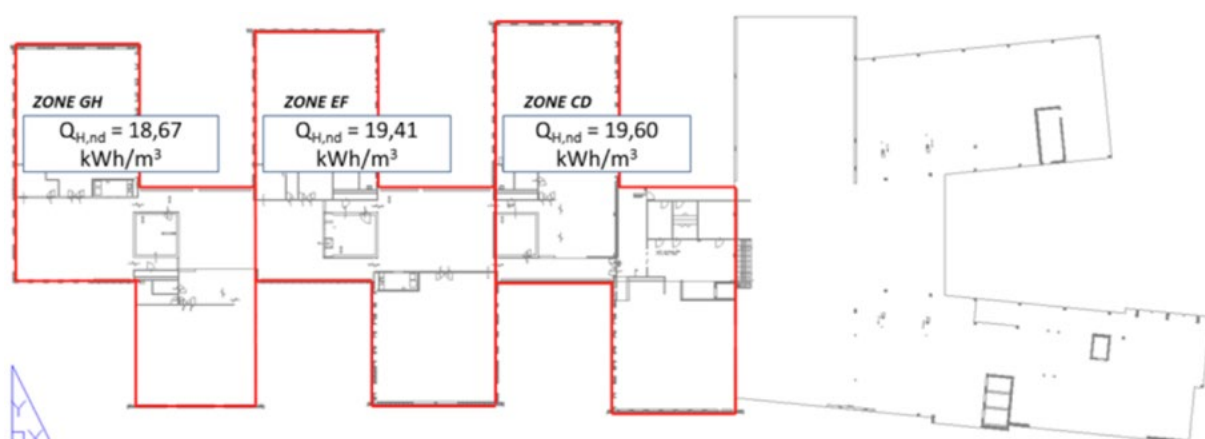
Figure 6. Building plan of the Zaanstad Town Hall with the indication of the building zones and their energy rating.
